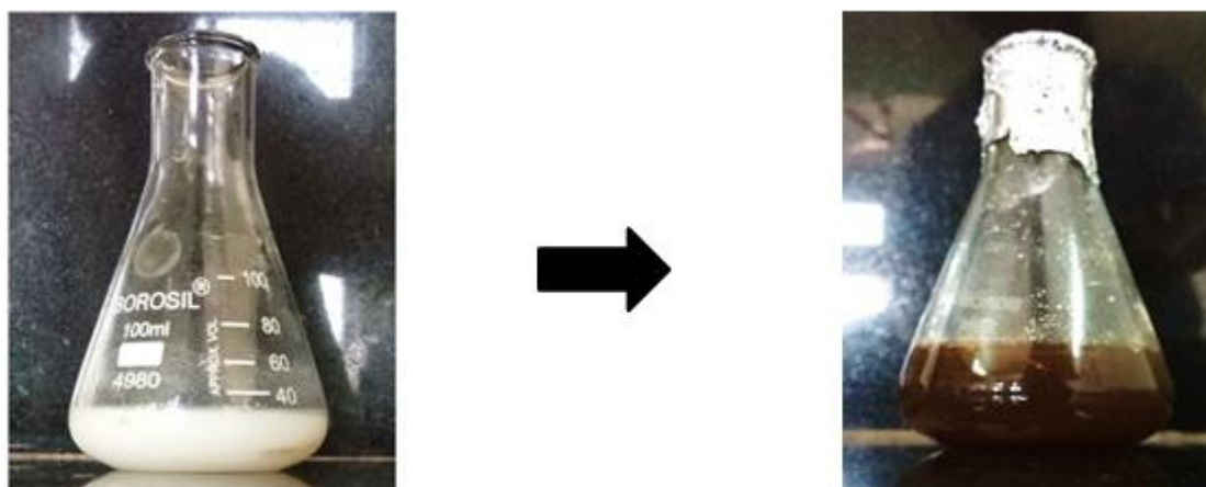
Figure 1: Change in color of the Euphorbia umbellata latex extract after addition of silver nitrate.
