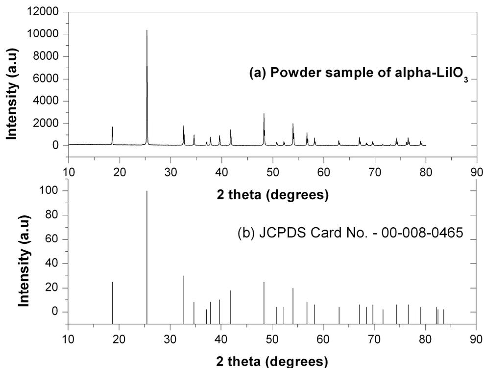
**Fig. 2** The pattern of X-ray powder diffraction: (a) powder sample pattern, (b) the standard JCPDS pattern
