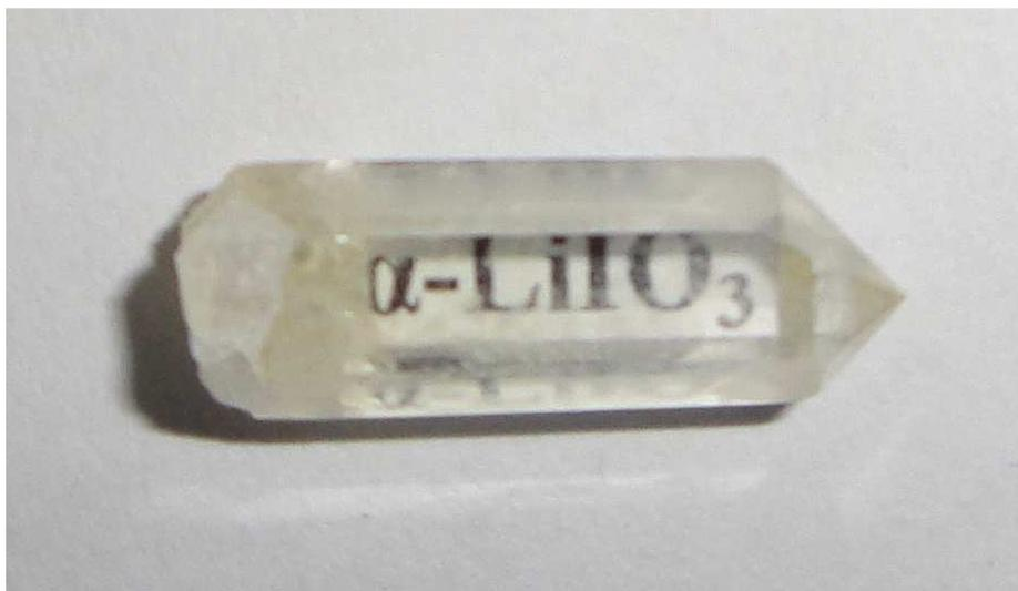
**Fig.1 As grown crystal of alpha-lithium iodate**
