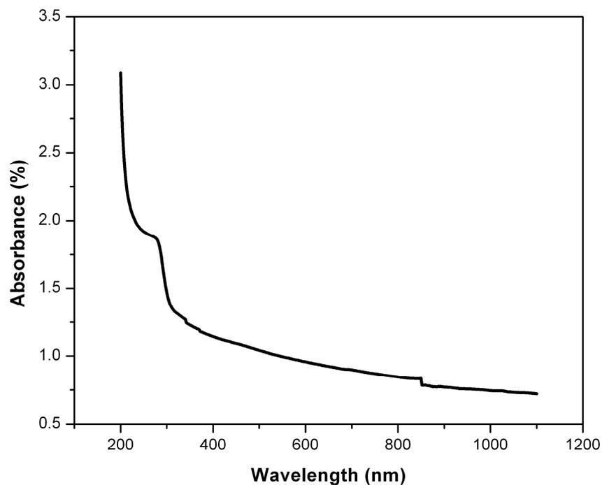
**Fig.3** Absorbance spectrum of alpha-lithium iodate
