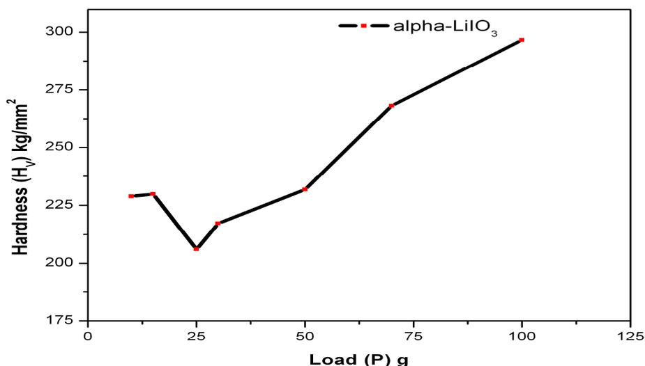
**Fig. 5** Microhardness studies of alpha-lithium iodate
