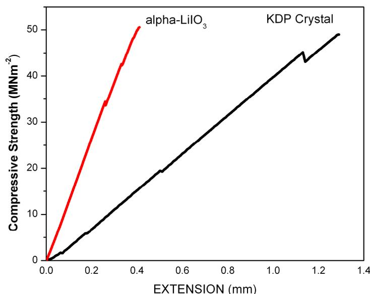
**Fig.4 Compressive strength of alpha-lithium iodate and KDP crystal.**
