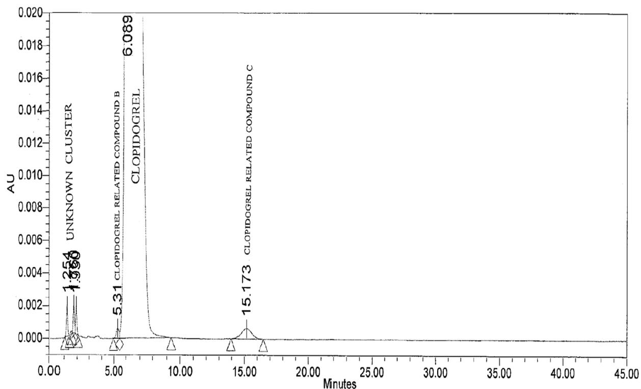
Fig- 2.d. 3 Month stability sample Chromatogram by USP method
