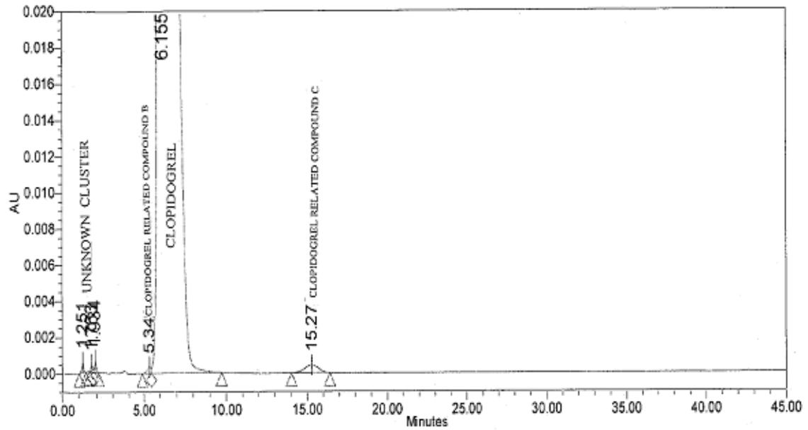
Fig- 2.b. 1 Month stability sample Chromatogram by USP method
