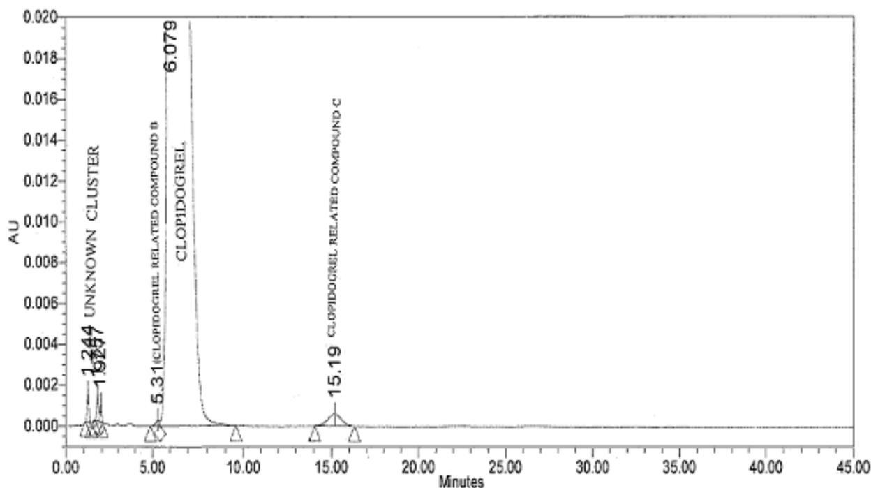
Fig- 2.c. 2 Month stability sample Chromatogram by USP method
