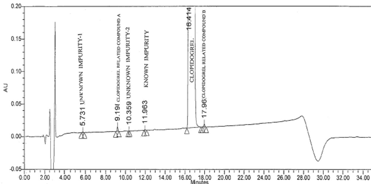
**Fig- 3.a. Initial sample Chromatogram by newly developed method**
